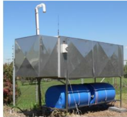
1500 L dual flow loop, two filter radon detector
