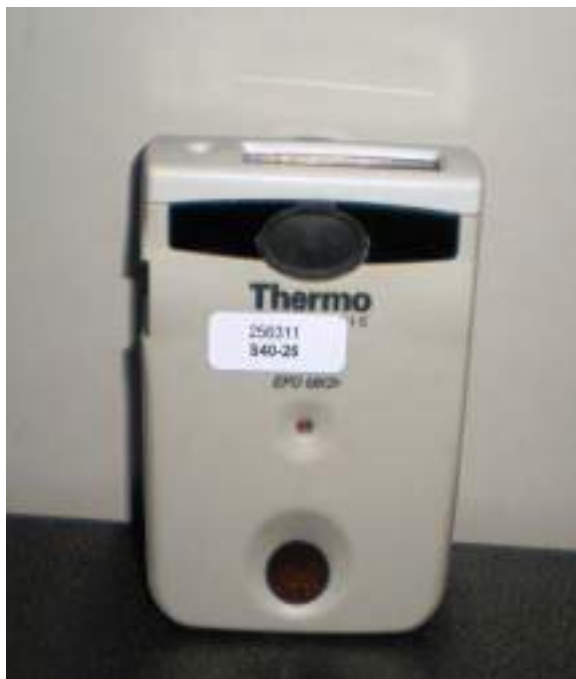
Figure 1: Example of a dosimeter with the label added by the coordinator. "S40" is the code to identify the dosimetry system (note: for presentation of the results, a different code was used). "26" is the code to identify a specific radiation quality, angle and dose range combination from the irradiation plan.
