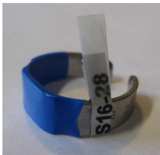
Figure 1. Example of a ring dosimeter with the label added by the coordinator. "S16" is the code to identify the dosimetry system (note: for presentation of the results, a different code was used). "28" is the code to identify a specific radiation quality, angle and dose range combination from the irradiation plan.
