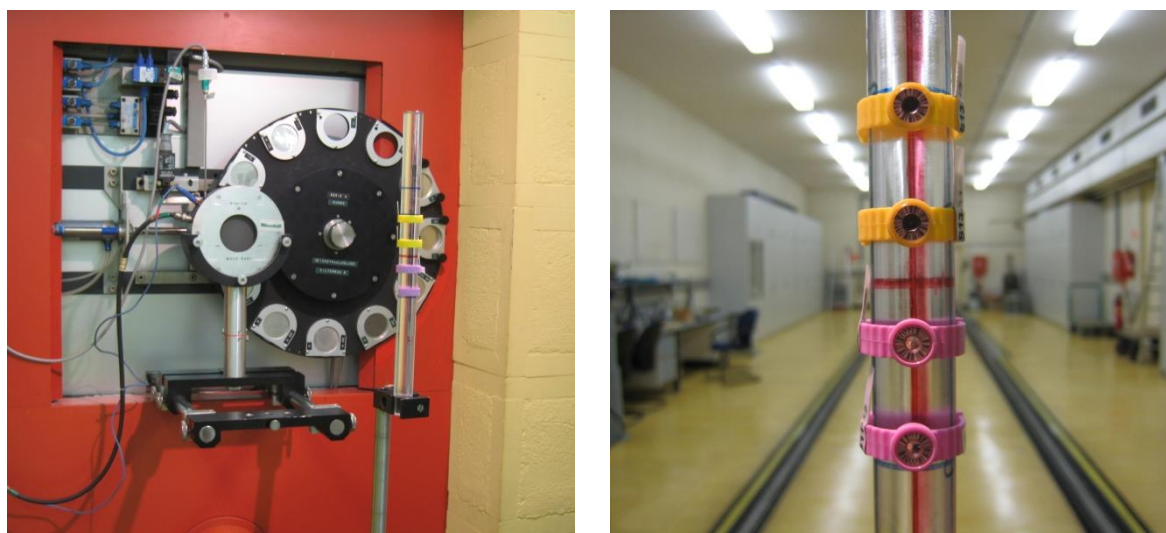
Figure 7: Irradiation set-up of finger ring dosimeters positioned on the ISO rod phantom in front of the MG320 X-ray facility at the accredited reference dosimetry laboratory of the Seibersdorf Laboratories (Austria).
