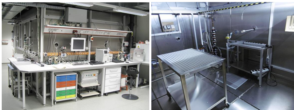
Figure 3.4 PAEC calibration chamber at the BfS Radon calibration laboratory.
