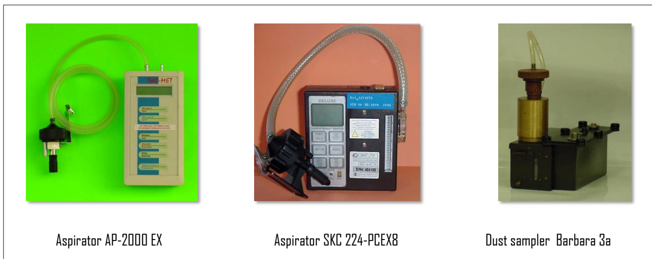
Figure 3.10 Integrating measuring devices for measurement of the potential alpha energy concentration.
