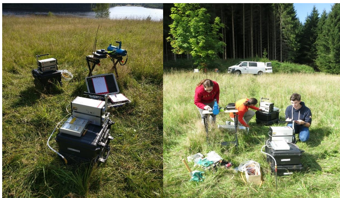
Figure 3.7 Taking a sample for soil gas radon measurements.
