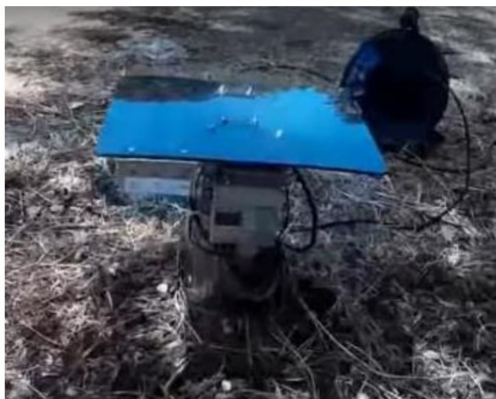
Figure 4.3 Continuous RADon Flux (CORAF) monitor designed and build at the INTE-UPC.
