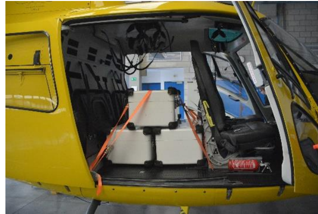
Two four liter NaI detectors (50 kg) Third contains electronics + battery (30 kg) Notebook PC and a small USB GPS
