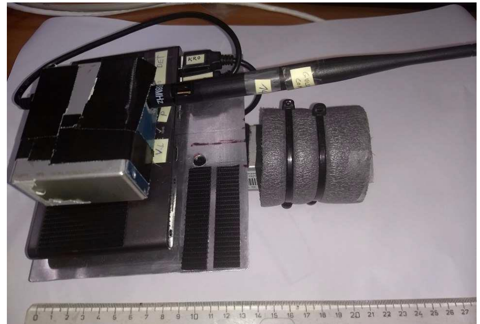
2"x1"x1" CsI detector (Kromek Sigma50) a small Windows10 PC and a device for long range radio transmission (700 grams)
